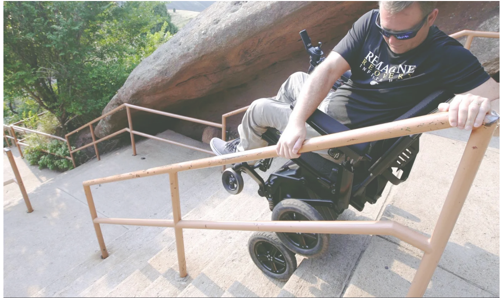
iBOT user Gary Linfoot stair climbs at Red Rocks, in Colorado. (Photo: Mobius Mobility)
